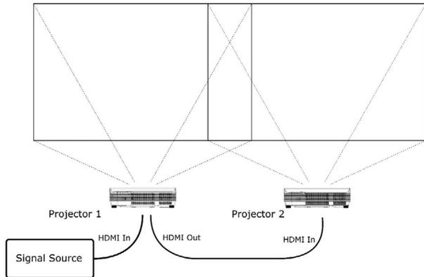
The part of the image output from the signal source using two projectors, surrounded by the red frame shown below, is displayed.
