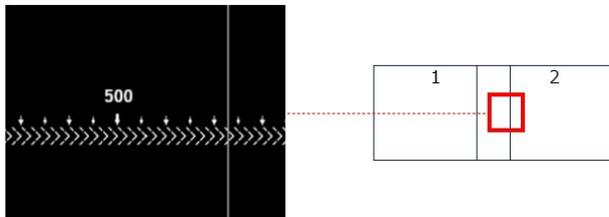
The left projector's scale is oriented in the opposite direction, allowing the overlap width to be measured in the same manner.
