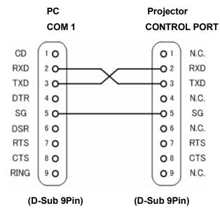
Connect COM port of the computer to CONTROL PORT of the projector.
