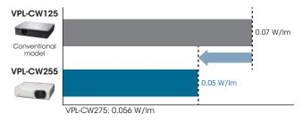
Power consumption efficiency (Lamp wattage (W) / Brightness (Im))
