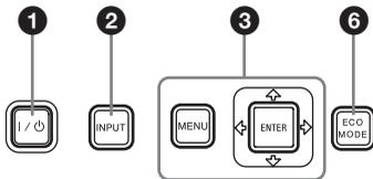
**1 Turning on the power/Going to standby mode**
