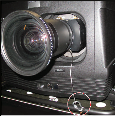
Image 1-11: Example using the bottom carrying handle on an HDX
