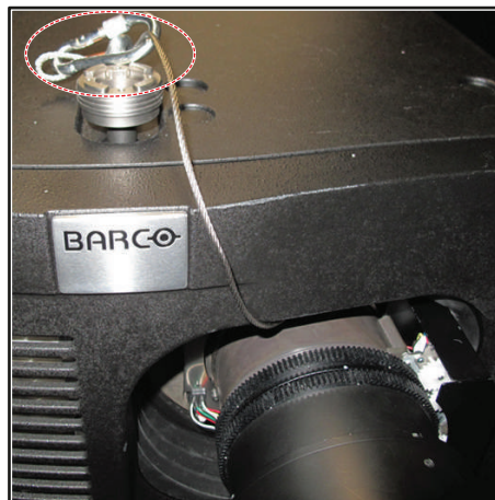
Image 1-16: Example using the hoisting eye
