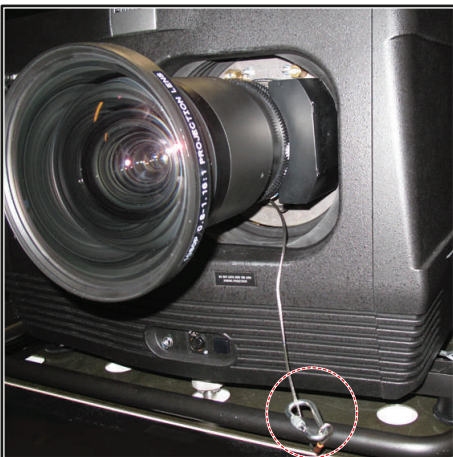
Image 1-15: Example using the bottom carrying handle
