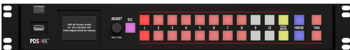
Image 4-3 Status screen and front-panel buttons
