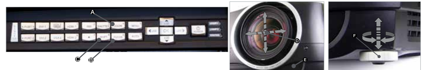
A: Zoom B: Focus C: Shift Press to activate. Adjust with arrow keys.
