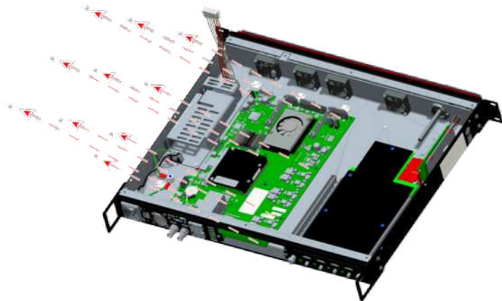
Image 16-20: Motherboard removal –motherboard screws
