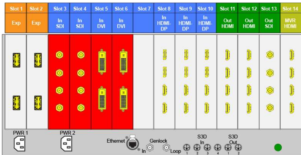
Image 6-15: E.g. E2 with an empty input-card slot
