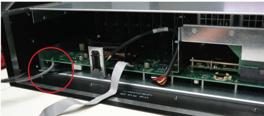
Image 15-35: USB Ext Cable connected to the Motherboard
