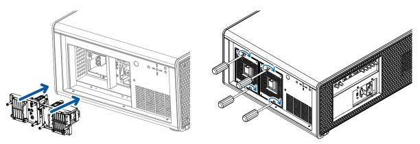
7. Replace the lamp cover and firmly secure the four screws on the lamp cover.
