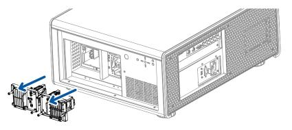
6. Insert the new lamp in the direction shown in the illustration into the lamp assembly; tighten the two screws using a screw diver and make sure the lamp is firmly secured to prevent the lamp from shaking or poor contact.
