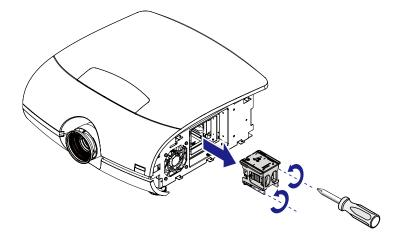
5. Insert the new lamp in the direction shown in the illustration into the lamp assembly; tighten the two screws using a screw diver and make sure the lamp is firmly secured to prevent the lamp from shaking or poor contact.
