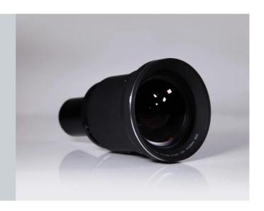
The EN76 lenses are designed specifically to maximize brightness, eliminate dust contamination, and to withstand motion and vibration through an improved barrel design. The lens consists of 20 glass elements with different coatings for the most demanding high-resolution performance, as well as being optimized for night vision and IR transmission. Additionally, to seal off unwanted air flow through the projector's front, through the grooves along the lens, a dust sealing has been designed.
