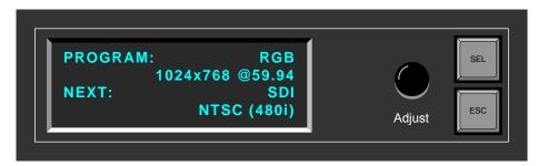
Figure 2-2. Display Section with sample Status Menu
