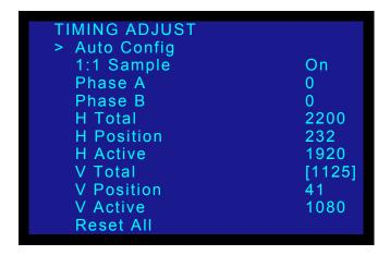
Figure 4-13. Timing Adjust Menu (sample)
