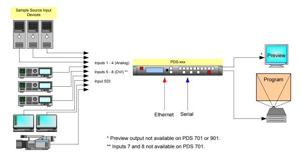
Figure 1-1. Block diagram, PDS system
