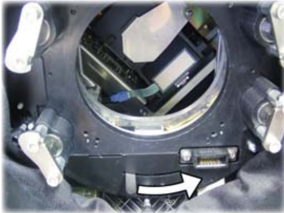
Image 2-2 Engage the lens locking system
