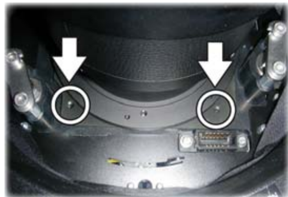
Image 2-4 TLD lens: locking top screws
