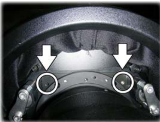
Image 2-3 TLD lens: locking top screws
