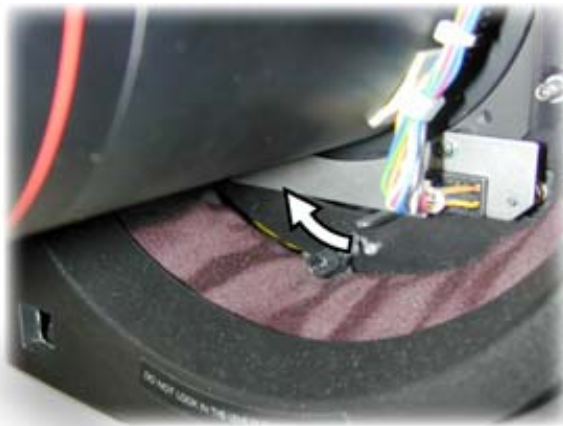
Image 2-1 Move the handle of the lens locking system to the left
