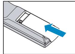
Note1: Be sure to insert the batteries in the corresponding orientations to match the polarities.
