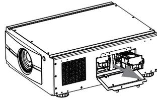
5. Insert the new lamp in the direction shown in the illustration into the lamp assembly; tighten the two screws using a screw driver and make sure the lamp is firmly secured to prevent the lamp from shaking or poor contact.
