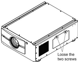
3. Use a screw driver to loosen the screws as shown in the illustration.
