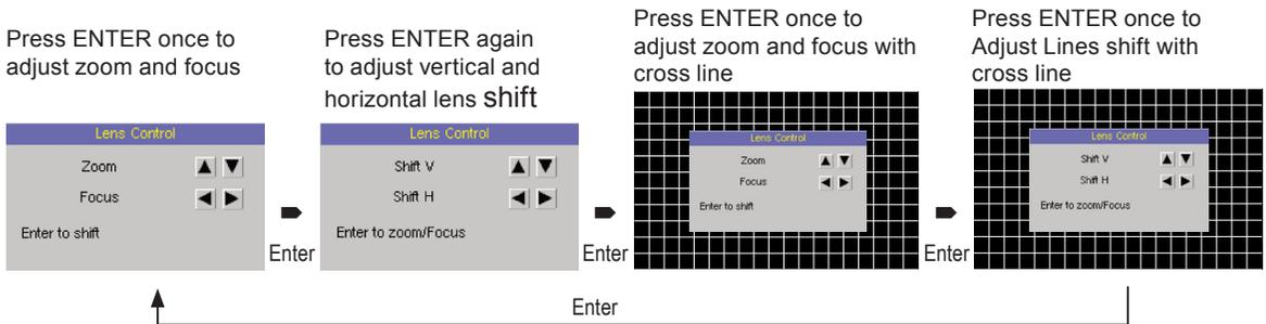
Method 2: Press the **MENU** button on the remote control and choose Alignment → Lens Control; then use the **▼▲▶◀** buttons to adjust the horizontal or vertical position of the lens.
