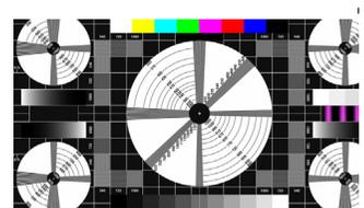
It is recommended that when adjusting the image, the horizontal total should be adjusted before the horizontal phase. However, if the image still flickers even after you have adjusted both, try lowering the image noise.
