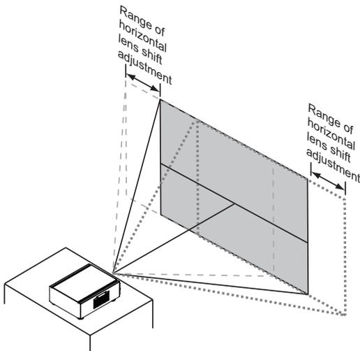
This illustration shows normal horizontal lens shift without the use of special specification lens or projector.
