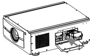
6. Replace the lamp cover and firmly secure the two screws on the lamp cover.
