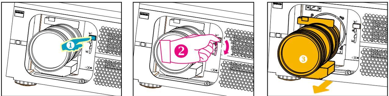
Make sure to hold the lens lever fully when install the lens (or remove the lens)
