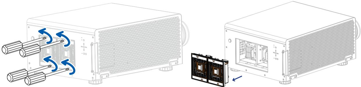
3. Use a screw driver to loosen the screws as shown in the illustration.
