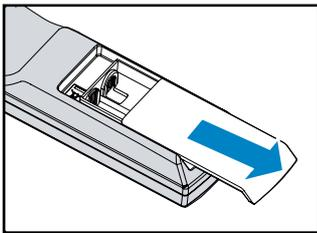
Insert two new AAA batteries (observe the polarity).
