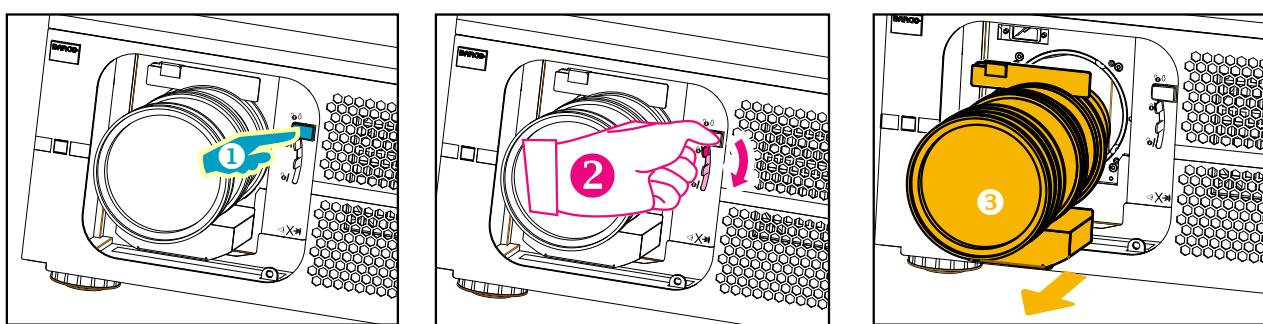
Make sure to hold the lens lever fully when install the lens (or remove the lens)
