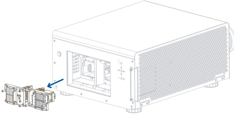
5. Insert the new lamp in the direction shown in the illustration into the lamp assembly; tighten the two screws using a screw driver and make sure the lamp is firmly secured to prevent the lamp from shaking or poor contact.
