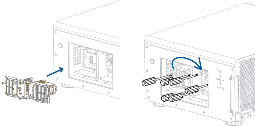
6. Replace the lamp cover and firmly secure the two screws on the lamp cover.
