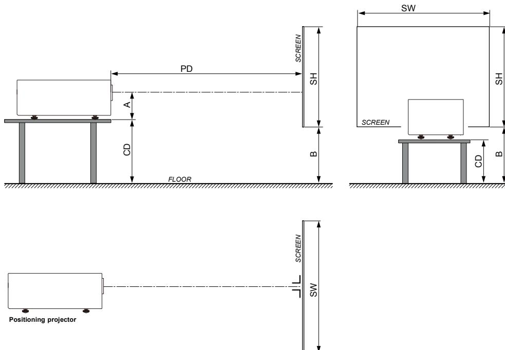
The projector should be installed at right angles (horizontally and vertically) to the screen at a distance PD. Note the distance (A) between lens centre and table surface is slightly variable. This distance (A) is nominal 14 cm in case all feet are turned in completely and the vertical lens shift is set to zero (0).
