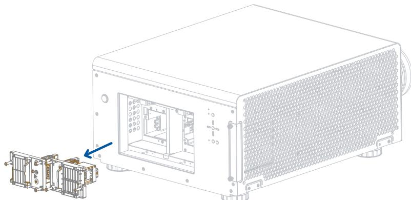
5. Insert the new lamp in the direction shown in the illustration into the lamp assembly; tighten the two screws using a screw diver and make sure the lamp is firmly secured to prevent the lamp from shaking or poor contact.
