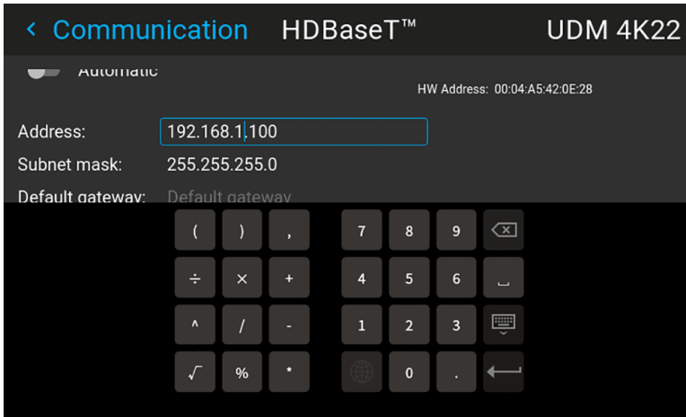
Image 10–18 Example of entering the IP address
