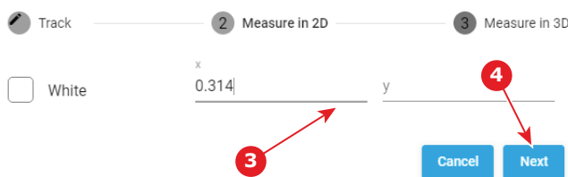
Image 9-5 White Point calibration - 2D measurement
