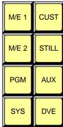
The term “**Memory Modules**” itself refers to the eight yellow buttons in the control panel’s **Memory Section**, and the corresponding columns in the Memory Menu’s table of registers. These buttons select the large categories of switcher functions to be included in the selected store or recall operation.
