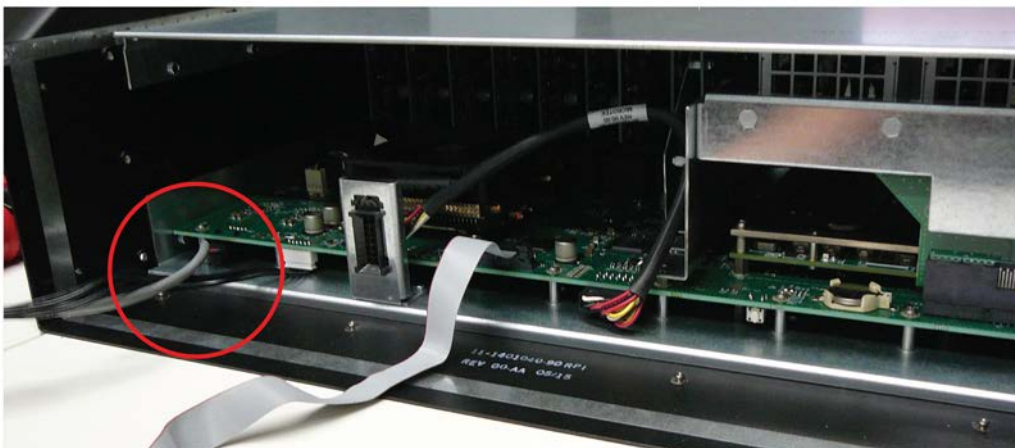
Image 15-35: USB Ext Cable connected to the Motherboard
