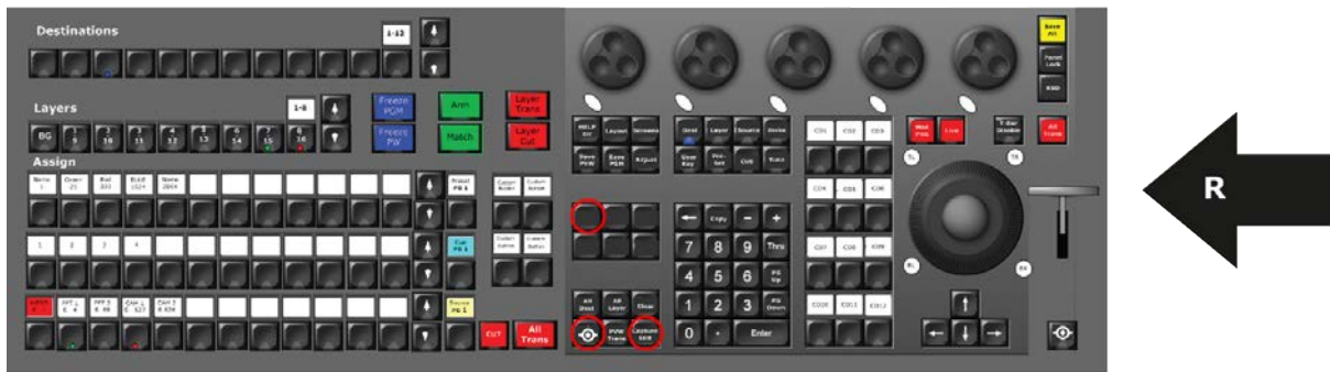
Image 12-3: EC-200/EC-210 CPU-reboot key combination
