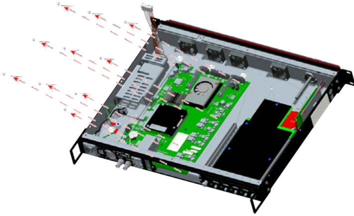
Image 16-20: Motherboard removal –motherboard screws
