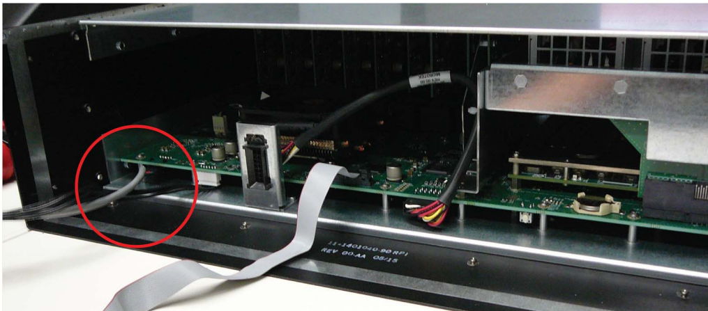
Image 15-35 USB Ext Cable connected to the Motherboard
