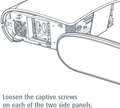
Loosen the captive screws on each of the two side panels.
