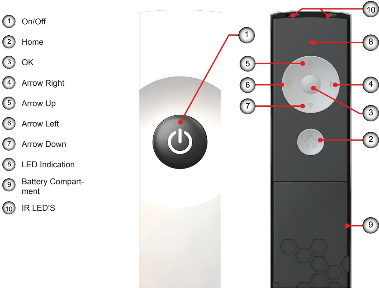
**Use the remote control to control these functions.**
