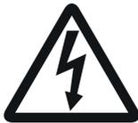
The lightning flash with arrowhead symbol within an equilateral triangle is intended to alert the user to the presence of uninsulated "dangerous voltage" within the product's enclosure that may be of sufficient magnitude to constitute a risk of electric shock.
