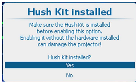
Image 2-12 Confirm Hush Kit physical installation.
