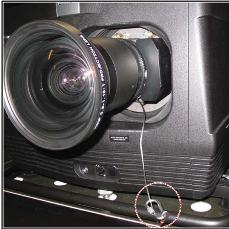
Image 3-29 Example using the bottom carrying handle
