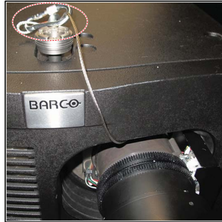
Image 3-30 Example using the hoisting eye
