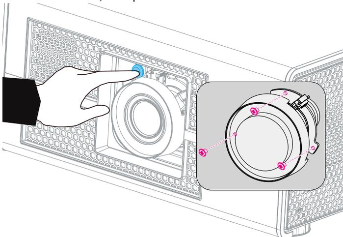
2. Counterclockwise rotate the lens to the end then you can follow the forward direction to remove the lens.
