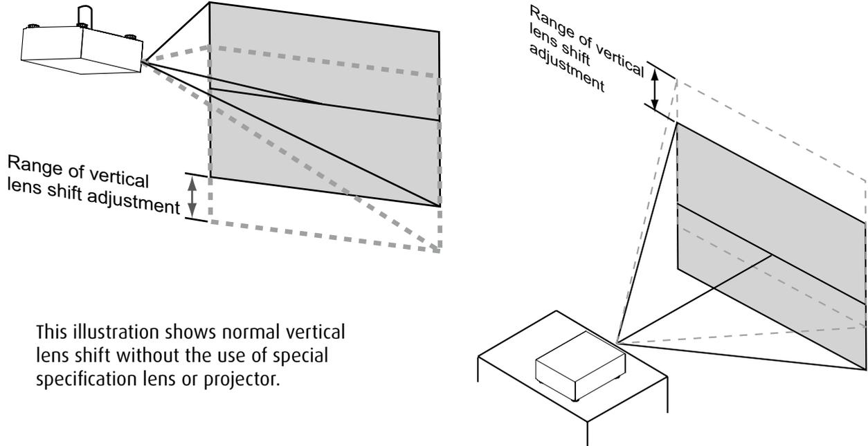
This illustration shows normal vertical lens shift without the use of special specification lens or projector.
