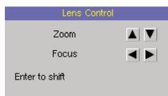
Press ENTER again to adjust vertical and horizontal lens shift
