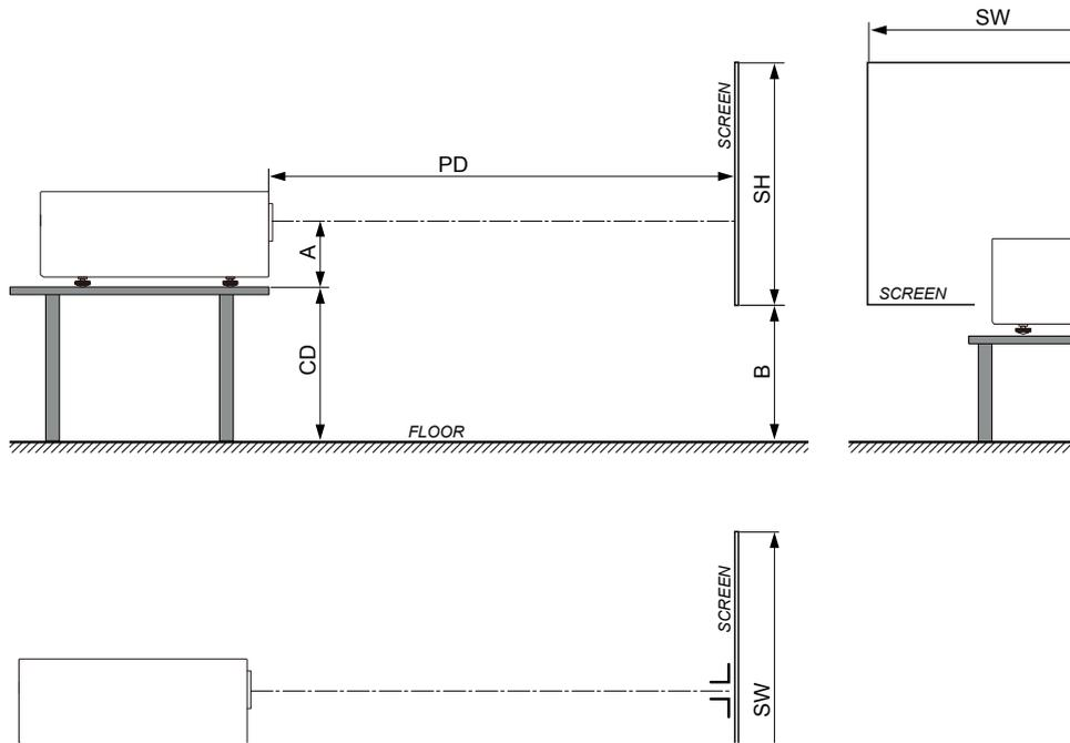
The projector should be installed at right angles (horizontally and vertically) to the screen at a distance PD. Note the distance (A) between lens center and table surface is slightly variable. This distance (A) is nominal 14 cm in case all feet are turned in completely and the vertical lens shift is set to zero (0).
