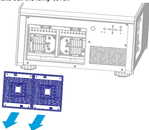
4. Use a screw driver to loosen the screws as shown in the illustration.
