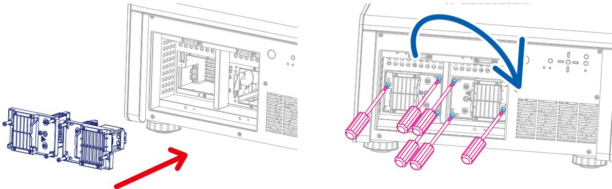
7. Replace the lamp cover and firmly secure the four screws on the lamp cover.
