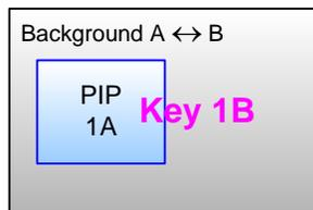
**Figure 1-8.** Single Mixer Effect 4 Diagram
