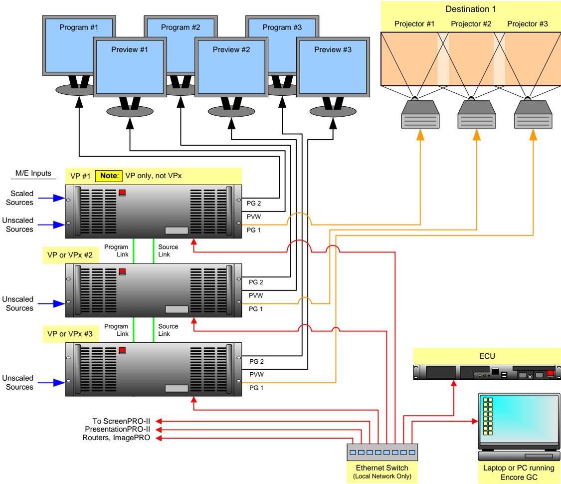
Figure 3-2. Sample Wide Screen Encore GC and ECU Configuration
