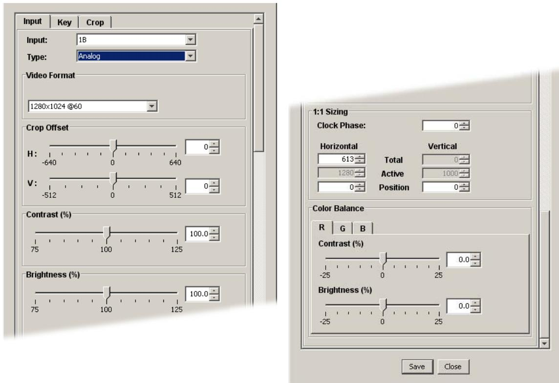
Figure 5-91. DSK Properties Dialog - Analog Type, Input Tab (sample)
