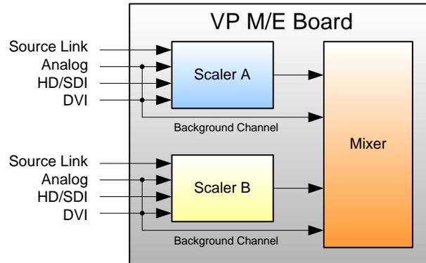
Figure 1-1. M/E Board Block Diagram, VP
