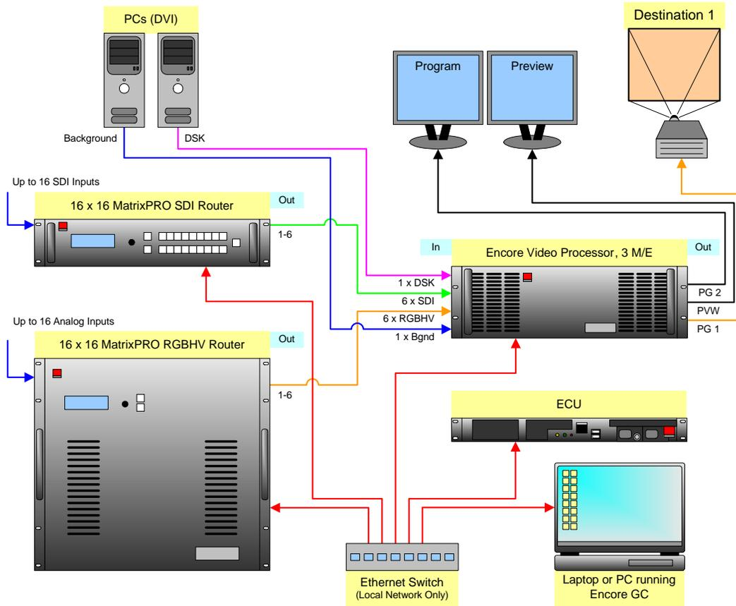
**Figure 3-1.** Sample Single Screen Encore GC and ECU Configuration
