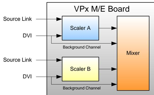
Figure 1-2. M/E Board Block Diagram, VPx
