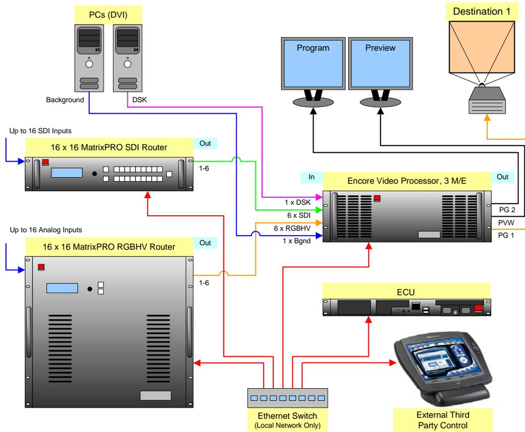
**Figure 1-18.** Sample externally controlled Encore GC and ECU system
