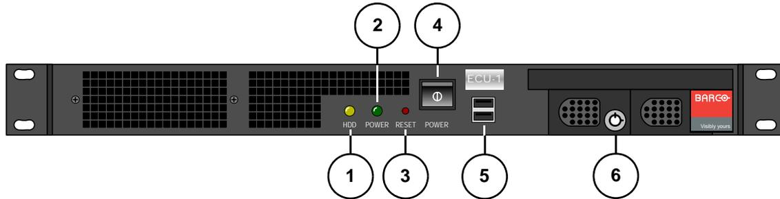
Figure 2-1. ECU front panel
