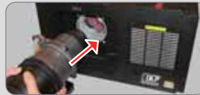
Slide lens in (motor connector on up side).
