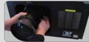
Make sure that motor connector is fully connected.
