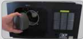
Removal of lens protection sponge.
