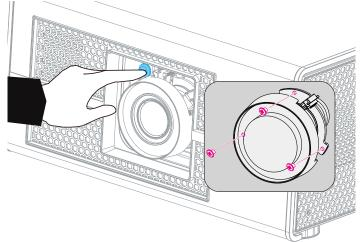
2. Counterclockwise rotate the lens to the end then you can follow the forward direction to remove the lens.
