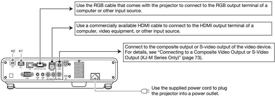
\*1 Use this port to connect a USB flash drive (page 23), a CASIO graphic scientific calculator (page 48), or the wireless adapter that comes with the projector (see the separate "Network Function Guide").
