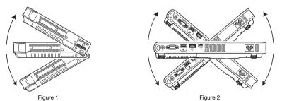
• With an XJ-M Series Projector, there is no limit on the vertical and horizontal setup angle.
