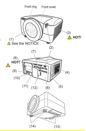
**► WARNING** ► HOT! : Do not touch around the lamp cover or the exhaust vents during use or just after use, since it is hot.
