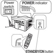
3. After making sure that the **POWER** indicator lights in steady orange, and press down the side marled "O" on the power switch.
