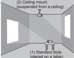
**NOTE** • In the case of ceiling mount, upward projection, or downward projection, the specified mounting accessories and service are required to install the projector. Request them from your dealer. Ask your dealer for installation other than styles above.
