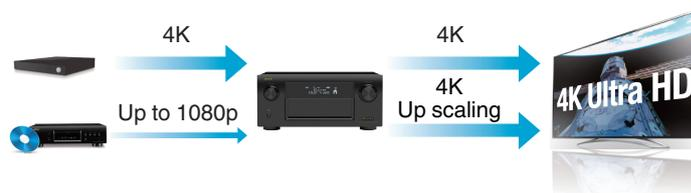
This unit is equipped with a 4K video upscaling function that allows analog video or SD (Standard Definition) video to be output via HDMI at 4K (3840 × 2160 pixels) resolution. This function enables the device to be connected to a TV using a single HDMI cable, and produces high definition images for any video source.
