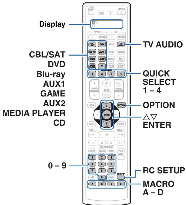
When preset codes are registered in the included remote control unit, it can then be used to operate any devices you have, such as DVD players or TVs made by different manufacturers.
