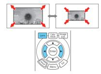
Press the **Lens** button on the remote control again and use the ▲, ▼, ◀, and ▶ buttons to reposition the image.
