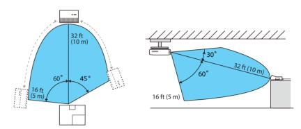
**Note:** Do not place the transmitter on a metal surface, as this may interfere with the signal. Make sure there are no obstructions between the transmitter and the projector.
