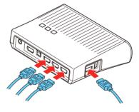
**Note:** You can connect tablets, smartphones, and other devices that support the MHL™ standard to the HDMI port on the side of the WirelessHD Transmitter. Some devices may require an adapter or may not require an MHL cable. Not all features or functions may be supported. Check your device's documentation for more information.
