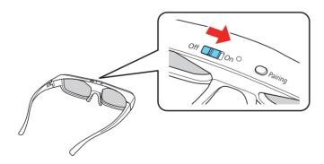
**Note:** If the glasses don't automatically display 3D content, you may need to pair them with the projector. Move the glasses within 10 feet (3 m) of the projector, then press and hold the **Pairing** button on the 3D glasses for at least 3 seconds. The status light on the glasses will alternately flash green and red, then remain green for 10 seconds if pairing is successful.
