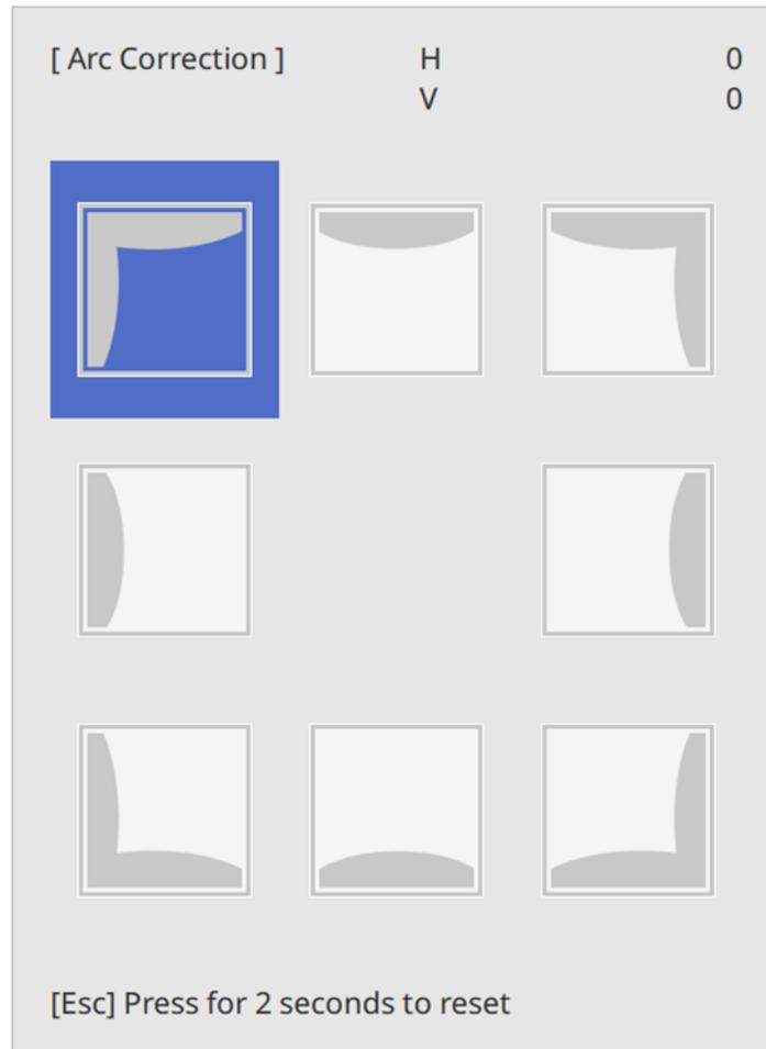
**Note:** To reset your adjustments, press the **Esc** button for at least 2 seconds to display a reset screen, and select **Yes**.
