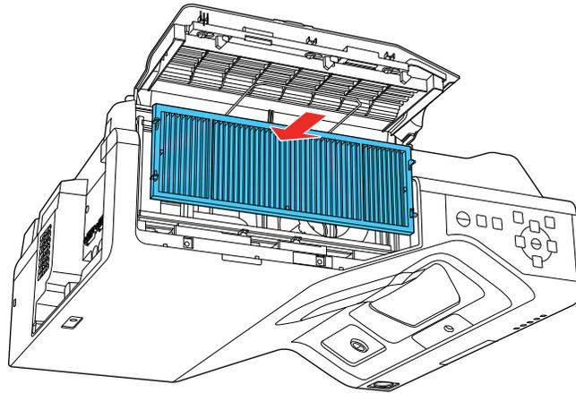
5. Close the air filter cover and slide the latch.
