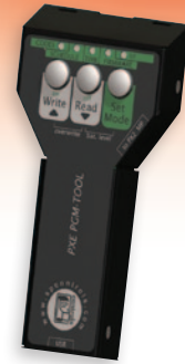
PXE-PGM-Tool Programming wand
