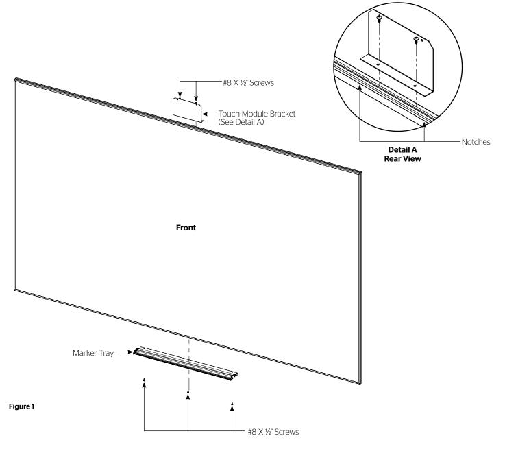
**Determining Screen Placement:** When installing the IDEA Screen with BrightLink projectors, you must leave at least 22" (56 cm) of space between the top of the screen and the ceiling to accommodate the projector wall mount.
