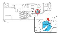
**3** Connect the streaming device to the projector's HDMI extension cable.
