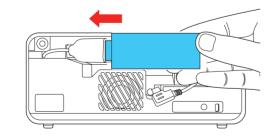
**4** Connect the USB power cable to the streaming device and fit the device securely inside the projector.
