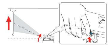
Move the focus lever on top of the projector left or right to adjust the image sharpness.
