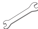
Open-ended wrench 13 mm (for M8 and M6) x 6 mm (for hexagonal shaft)
