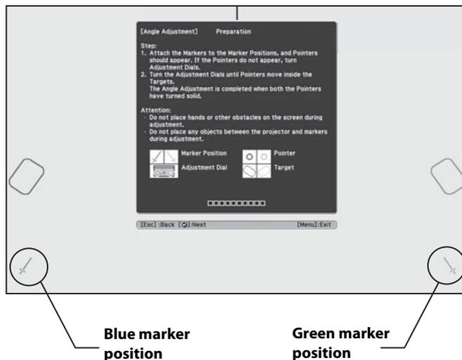
Match the positions so that the crosses (①) overlap with the points (②) on the marker positions (↖) (↘). Move the marker over the projected cross until the lines of the cross align with the lines on the marker.
