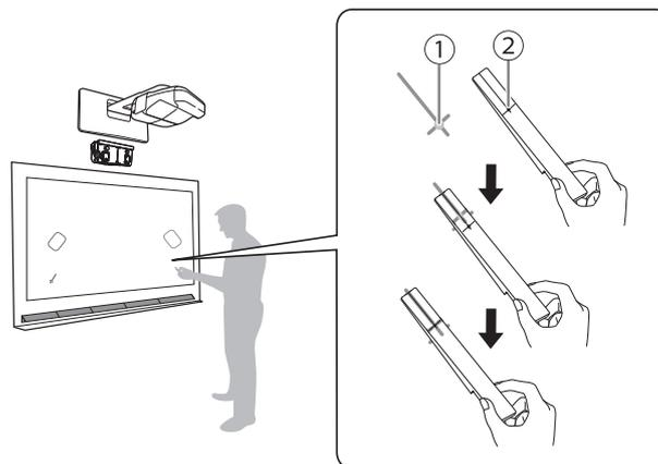
When circles ○ with the same color (blue and green) as the marker positions are displayed on the left and right of the projection screen, attach the markers to the projection screen as follows:
