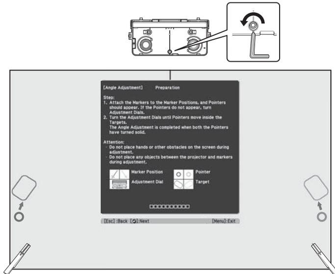
Tightening the adjustment screw moves the pointers diagonally down away from the center of the projected image.
