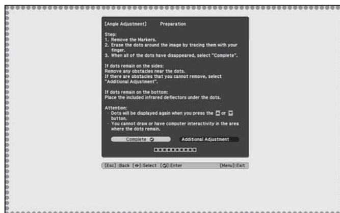
16. Trace the dots with your finger as shown. When angle adjustment is performed correctly, the traced dots disappear.
