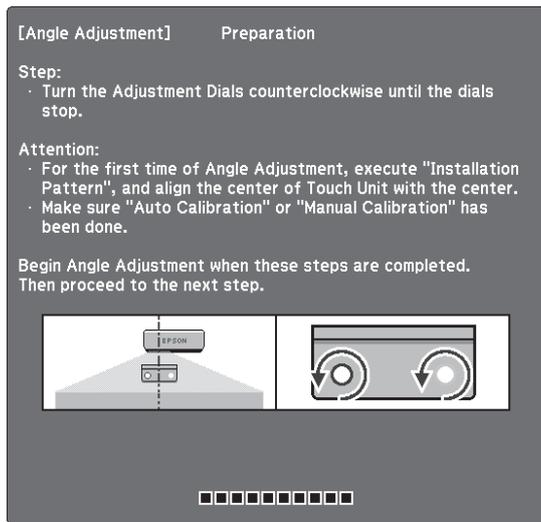
6. Turn the adjustment dials on the Touch Unit counterclockwise until you hear a click. Then, press the button on the remote control.
