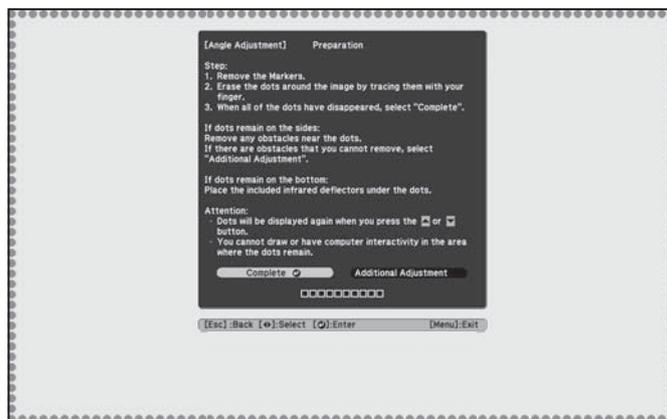
13. Trace the dots with your finger as shown. When angle adjustment is performed correctly, the traced dots disappear.
