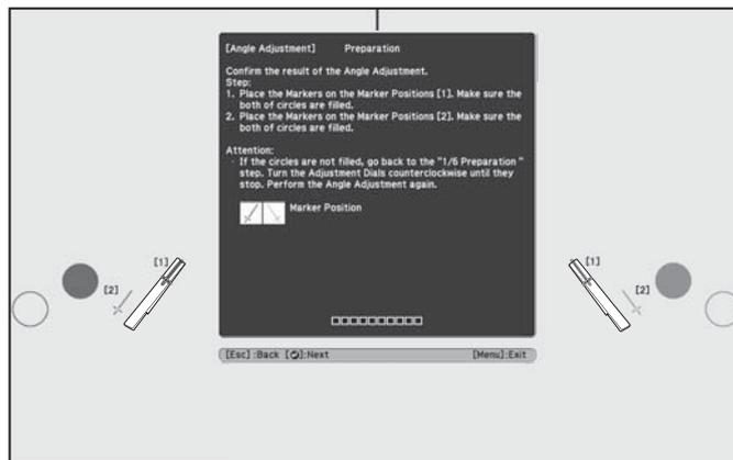
11. Place the markers at the bottom marker positions [2]. When angle adjustment is performed correctly, the bottom circles become solid (●). If the bottom circles do not become solid (●), start again from step 4.
