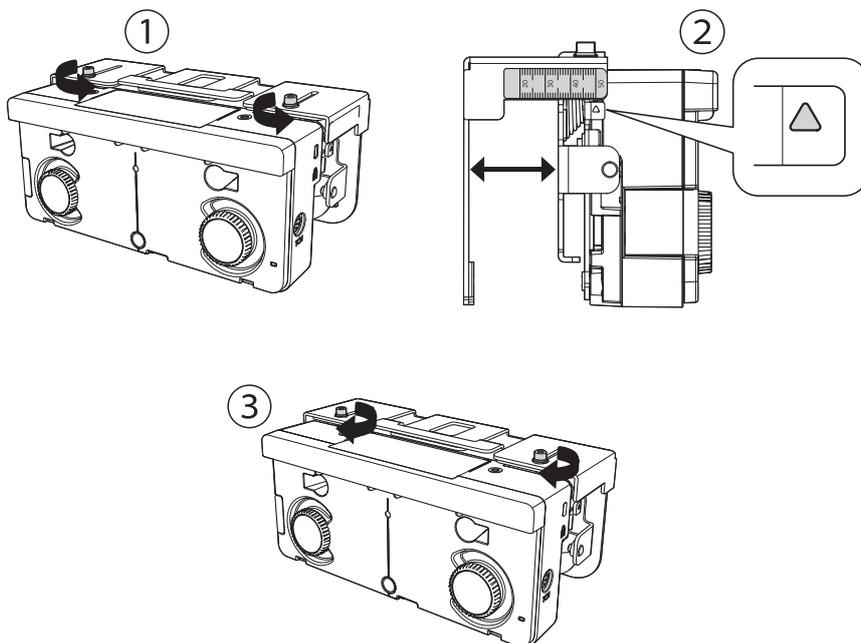
6. Insert the M4 × 55 mm or M4 × 70 mm hexagon socket head cap bolt into Touch Unit and tighten the bolt until the Touch Unit is parallel to the installation plate.
