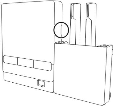
If you are using the Touch Unit, make sure that you do not install the Control Pad or Pen Stand in the shaded areas of the following figure. The Touch Unit will not operate correctly if anything is obstructing the infrared signal.
