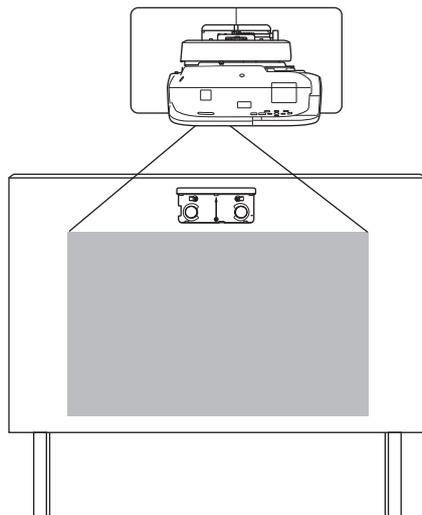
Make sure there are no obstacles, such as cables, or protruding objects such as whiteboard trays, pen holders, or thick frames in the shaded areas in the following figure. The Touch Unit will not operate correctly if anything is obstructing the infrared signal.
