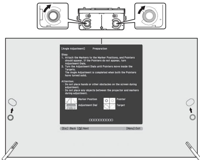
Turning an adjustment dial counterclockwise moves the pointer diagonally down away from the center of the projected image.
