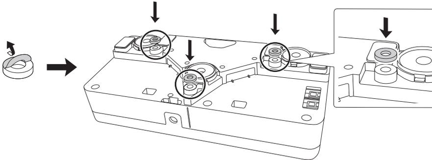
Secure the Touch Unit with three (3) M4 screws (not included).
