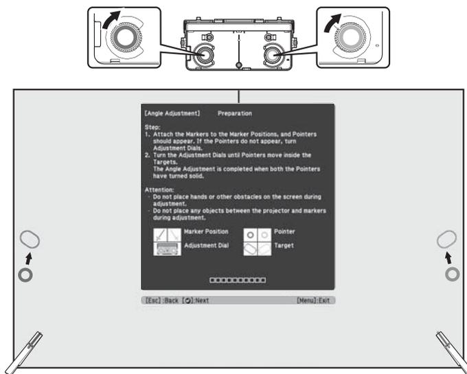
Turning an adjustment dial counterclockwise moves the pointer diagonally down away from the center of the projected image.
