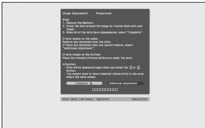
17. If there is an obstacle that cannot be removed, such as a whiteboard tray or frame, remove the tape from the back of the supplied infrared deflectors and stick them to the screen so that the laser is not reflected by the obstacle.
