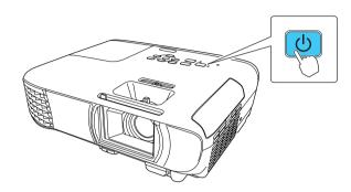
**Note:** To shut down the projector, press the  $\bigcirc$  power button twice.
