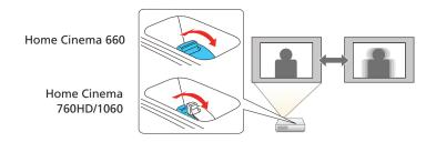
If your image looks like \_\_\_\_ or \_\_\_, you may have placed the projector off to one side of the screen at an angle. Place the projector directly in front of the center of the screen, facing the screen squarely. If you can't move the projector, use the horizontal keystone slider on the projector to correct the image shape.
