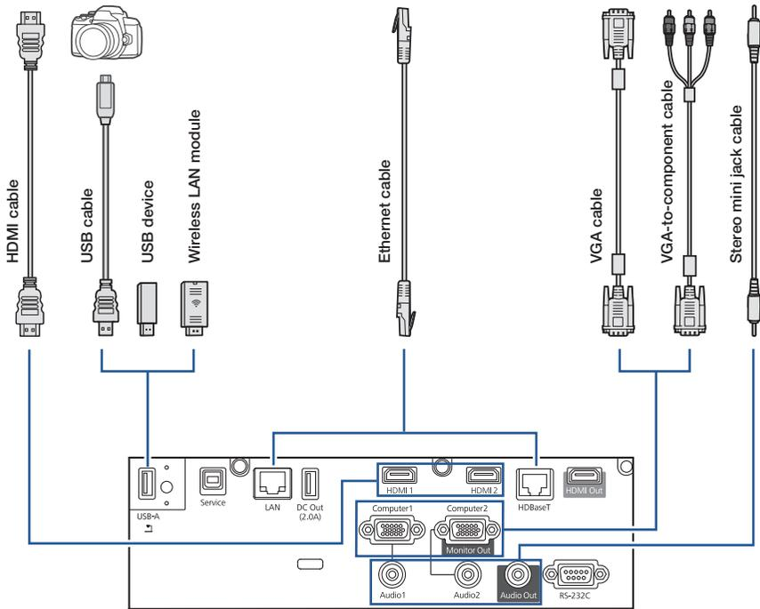
**Note:** The HDMI Out and DC Out ports are not available on the PowerLite EB-L520U.
