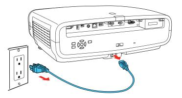
**Caution:** To avoid damaging the projector or laser, never unplug the power cord when the Status light is on or flashing.
