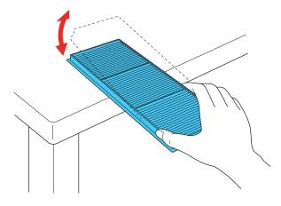
**Caution:** Do not use excessive force when tapping the air filter, or it may crack and become unusable. Do not rinse the air filter in water, or use any detergent or solvent to clean it. Do not use canned air; the gases may leave a residue, or push dust and debris into the projector's optics or other sensitive areas.
