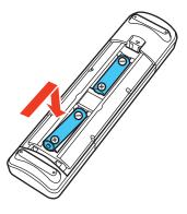
**Warning:** Make sure the batteries are inserted in the correct positions. If the batteries are not inserted correctly, they could explode or leak, causing a fire, injury, or damage to the product.
