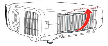
4. Pull the air filter out of the projector.
