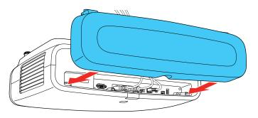
4. Tighten both cable cover screws.
