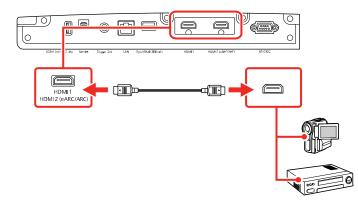
**Note:** When an audio/video source that meets the HDMI CEC standard is connected to the projector's HDMI port, you can use the projector's remote control to control certain features of the linked device by pressing the **HDMI Link** button on the remote control and setting **HDMI Link** to **On**.
