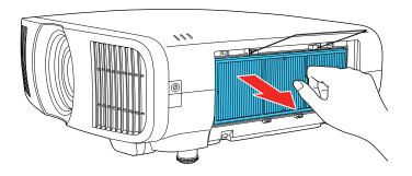
**Note:** Air filters contain polypropylene. Dispose of used air filters according to local regulations.
