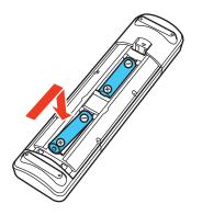
**Warning:** Make sure the batteries are inserted in the correct positions. If the batteries are not inserted correctly, they could explode or leak, causing a fire, injury, or damage to the product.
