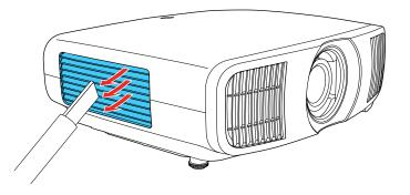
Note: Canned or compressed air is not recommended as it can blow dust into the projector.
