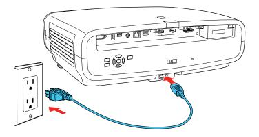
2. Plug the power cord into an electrical outlet.
