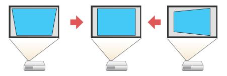
**Note:** Try adjusting the projector's placement and lens shift before using keystone correction. Digital image correction reduces the number of pixels in the image.
