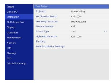
4. Select **Geometry Correction** and press [Enter]. You see the **Geometry Correction** screen.
