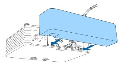
**3** Tighten the cable cover screws.
