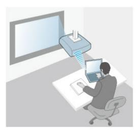
• Turning off simple AP mode lets you connect to smartphones, tablets, or computers over a wireless network access point. When you use this method, connect the projector using **Advanced Connection Mode** of the Epson iProjection software.
