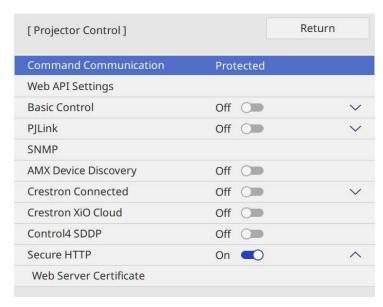
Set the **Crestron Connected** setting to **On** to allow the projector to be detected.
