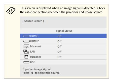
• Press the button for the source you want on the remote control. If there is more than one port for that source, press the button again to cycle through the sources.
