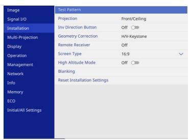
Select **Geometry Correction** and press [Enter]. You see the **Geometry Correction** screen.
