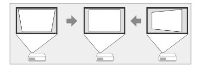
You can correct images up to 30° right, left, up, or down. (EB-L890E/EB-L895E/EB-L790SE/EB-L795SE/EB-L695SE/EB-L690E/EB-L890U/EB-L895U/EB-L790U/EB-L790SU/EB-L690U/EB-L690SU/EB-L695SU)
