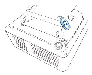
Attach the wire clamp to another carabiner, and then use the screw to fix the wire clamp to the wire clamp fixing point on the projector.
