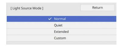
If you set the **Light Source Mode** setting to **Custom**, select **Brightness Level** and use the left and right arrow buttons to select the brightness.
