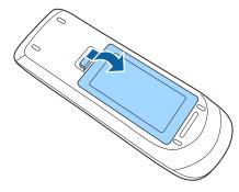
Remove the old batteries, if necessary.
