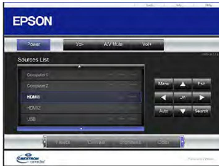
4. Select the input source that you want to control in the Sources List box. You can scroll through available sources using the up and down arrows in the box.
