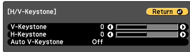
6. Use the arrow buttons on the projector or the remote control to select between vertical and horizontal keystone or balance correction and to adjust the image shape as necessary.
