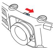
If the projector is on a table, you can level the image by turning any of the projector's adjustable feet.
