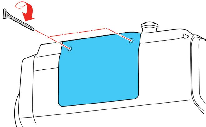
**Note:** Be sure the lamp cover is securely installed or the lamp will not come on.
