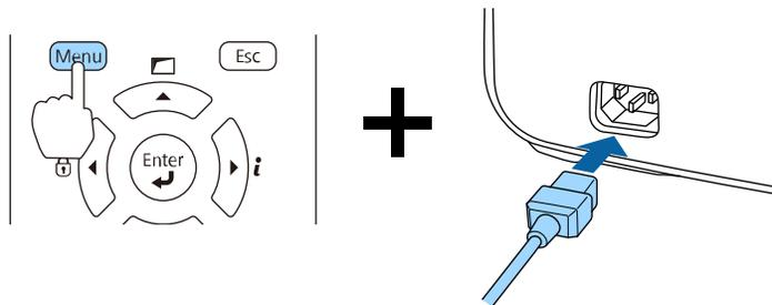
5. When the power and Status lights turn blue and the Lamp and Temp lamps turn orange, release the **Menu** button.
