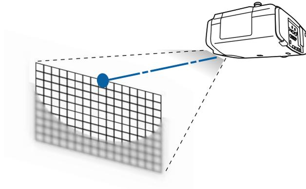
4. Rotate the distortion ring until the edges of the image are also focused.
