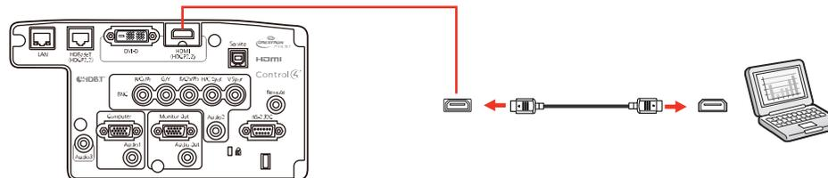
**Note:** The projector converts the digital audio signal sent from your computer into a mono analog signal for the internal speaker or a stereo analog signal if you are connecting to external speakers.
