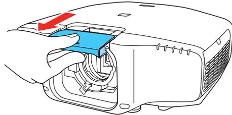
2. When using one of the following lenses, attach the lens connector cap: ELPLS04, ELPLU02, ELPLR04, ELPLW04, ELPLM06, ELPLM07, or ELPLL07.
