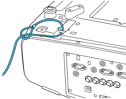
**Note:** Do not pass drop-prevention cables through the security cable attachment point when mounting the projector on a wall or ceiling.
