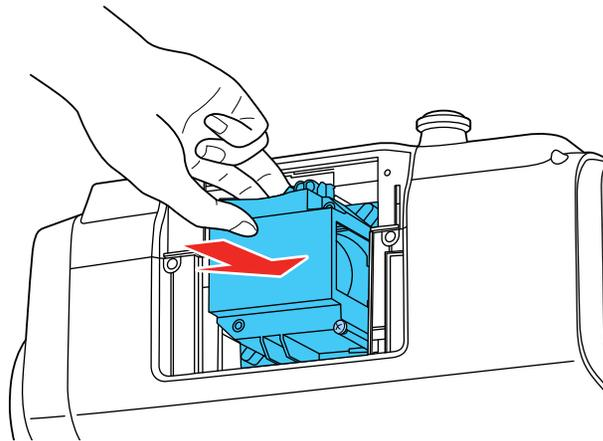
**Caution:** Do not touch any glass on the lamp assembly to avoid premature lamp failure.
