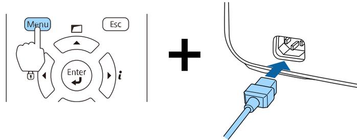
4. When the power and Status lights turn blue and the Lamp and Temp lights turn orange, release the **Menu** button.
