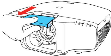
4. Hold the lens firmly as you slide the lock lever to the **Release** position (as shown) until you hear it click.
