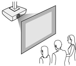
**Note:** Be sure to leave at least 20 inches (50 cm) of space in front of the air exhaust and intake vents and, when setting up multiple projectors, 20 inches (50 cm) of space between the projectors.
