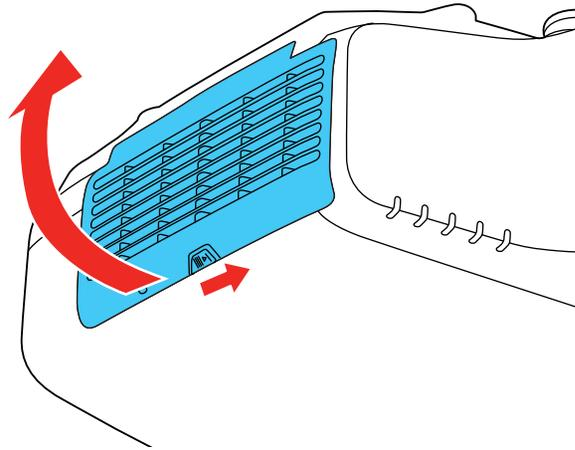
3. Pull the air filter out of the projector.
