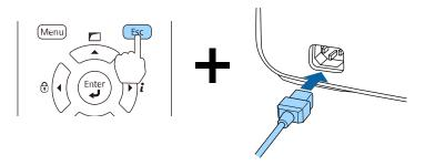
4. When the power and Status lights are blue and the Lamp and Temp lights are orange, release the **Esc** button.
