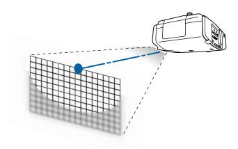
4. Rotate the distortion ring until the edges of the image are also focused.
