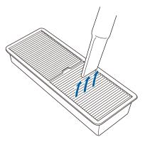
Note: If dust is difficult to remove or the air filter is damaged, replace the air filter.
