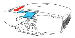
2. When using one of the following lenses, attach the lens connector cap: ELPLS04, ELPLU02, ELPLR04, ELPLW04, ELPLM06, ELPLM07, or ELPLL07.
