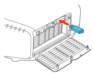
**Note:** Connect the flash drive directly to the projector. Do not use a hub or your settings may not be saved correctly.
