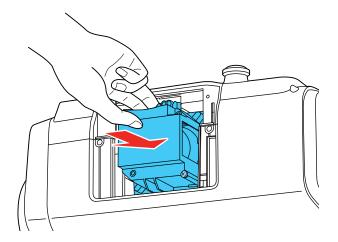
**Caution:** Do not touch any glass on the lamp assembly to avoid premature lamp failure.
