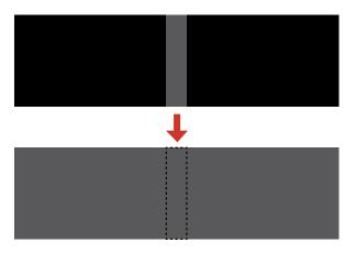
**Note:** You cannot adjust the black level when a test pattern is displayed. The brightness and tone of the overlapping areas may differ from the rest of the image even after adjusting the black level.
