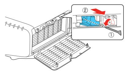
4. Insert the wireless LAN module into the port.
