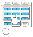
**Note:** If you don't know the projector's ID, hold down the **ID** button and press the **Home** button to temporarily display the projector's ID on the screen. If the batteries are left out of the remote control for an extended period, the remote control ID returns to its default setting.
