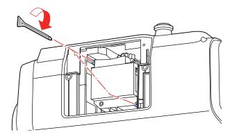
8. Replace the lamp cover and tighten the screws to secure it.
