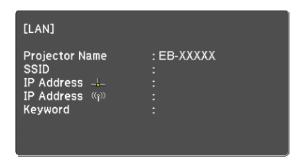
3. Verify that an SSID and IP address are displayed, then remove the wireless LAN module from the projector if necessary.
