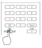
3. Hold down the **ID** button on the remote control while you press the numeric button that matches the projector's ID. Then release the buttons.
