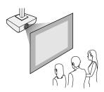
**Note:** Be sure to leave at least 20 inches (50 cm) of space in front of the air exhaust and intake vents and, when setting up multiple projectors, 20 inches (50 cm) of space between the projectors.
