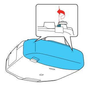
To remove the cover, loosen both screws and pull the cover off of the projector.
