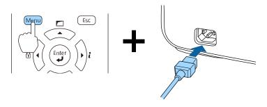
5. When the power and Status lights turn blue and the Lamp and Temp lamps turn orange, release the **Menu** button.
