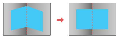
**Note:** For the best results, project from the front of the screen onto a right-angled surface with the lens centered horizontally using lens shift. The image may not be evenly focused throughout even after performing the steps here. If you are using the optional short throw lens (ELPLU01), you may not be able to adjust the Corner Wall setting.
