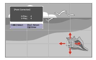
9. Use the arrow buttons to correct the image shape in all necessary directions.
