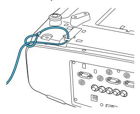
**Note:** Do not pass drop-prevention cables through the security cable attachment point when mounting the projector on a wall or ceiling.
