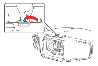
4. Insert the lens straight into the projector's lens socket with the white dot facing up.
