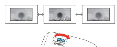
If your image looks like or , you've placed the projector off to one side of the screen at an angle. Place the projector directly in front of the center of the screen, facing the screen squarely. Or use the horizontal keystone slider on the projector to correct it.
